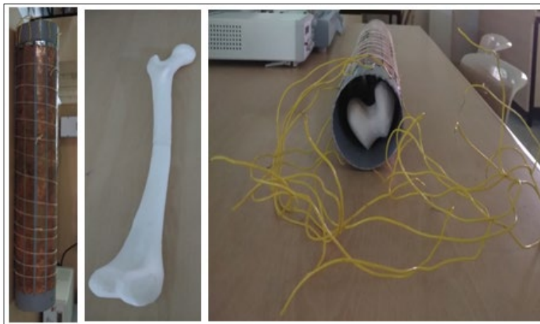
Figure 6. ECT sensor, Femur bone and ECT sensor with bone placed within it.
