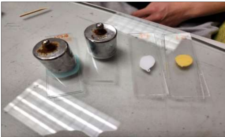
Figure 3. Presents the spreadability evaluation of toothpaste on a slide glass with standard weights.
