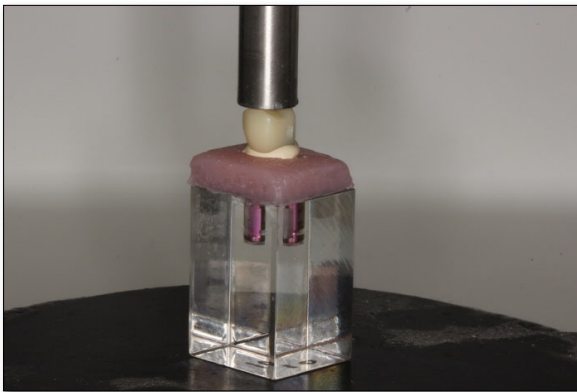
Figure 3. Crowns cemented under standard pressure by applying a 5 kg axial force for 10 min.
