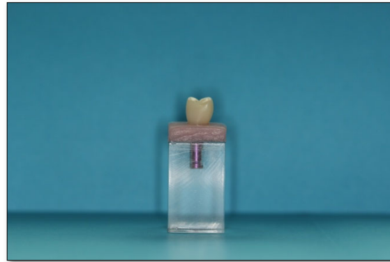
Figure 1. One of the test samples with the crown-abutment complex.
