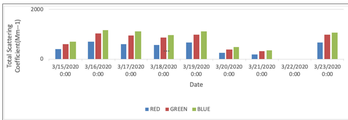
Figure 9. Daily mean variations in total scattering coefficient recorded with an Aurora 4000 Polar nephelometer at AUH during 15-23 March 2020 covering the Janata Curfew day on 22 March 2020.
