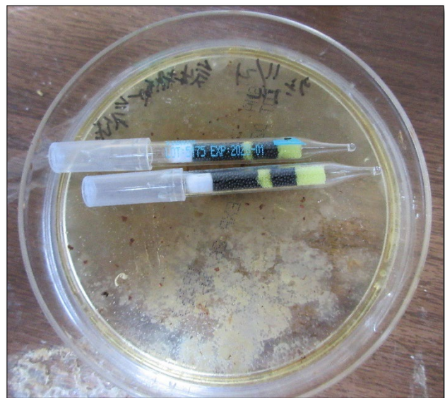
Figure 9. Photograph of the equipment used for gas assays. After gas collection, the tubes were sealed.
