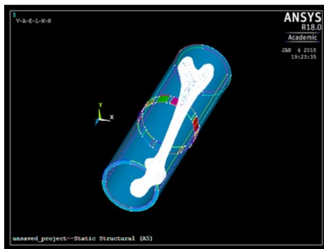
Figure 4. 3D model of sensor with bone in it.
