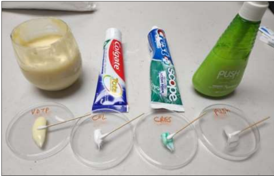
Figure 2. Presents the scratchiness test with Petri Dish and sterile cotton swabs on toothpaste samples.
