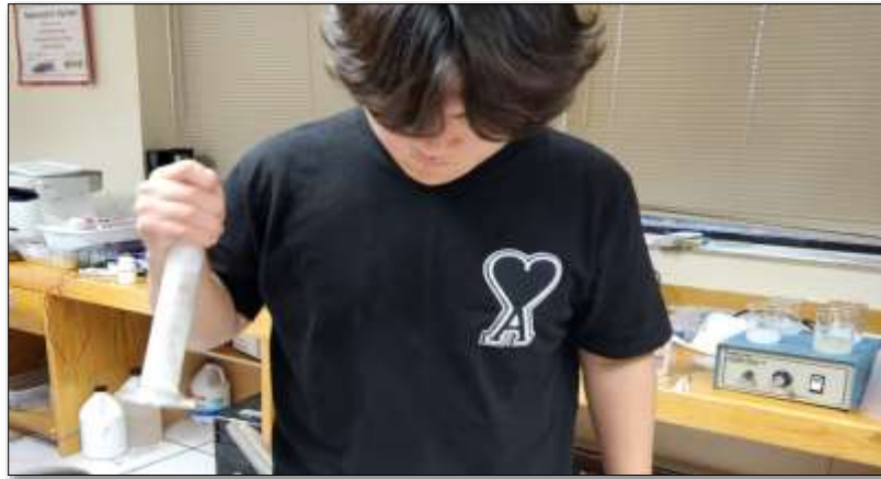
Figure 4. Presents the pictorial presentation of foaming tests by shaking a 100 mL graduated cylinder filled with toothpaste stock solution.
