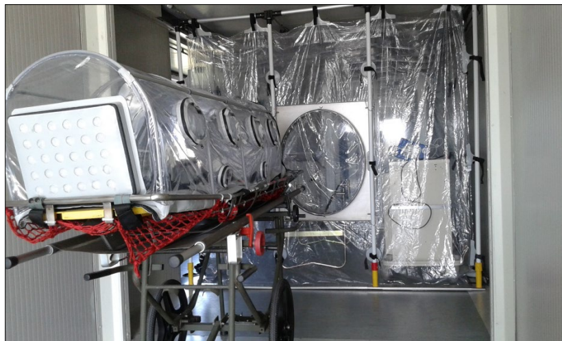
Figure 3. IsoArk N36-4 Isolation stretcher with HEPA filtration system and a Spinal board (yellow board) as support, upon ECO/NATO stretcher, in front of the Isolation Chamber Isoark equipped with Oblo' and CBRN filtration system [3].
