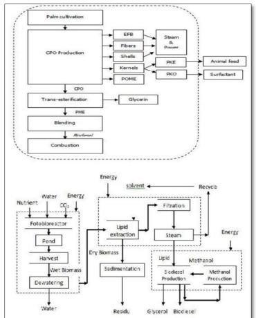
Figure 1. Scheme of biodiesel production from (a) Palm Oil and (b) Chlorophyceae.
