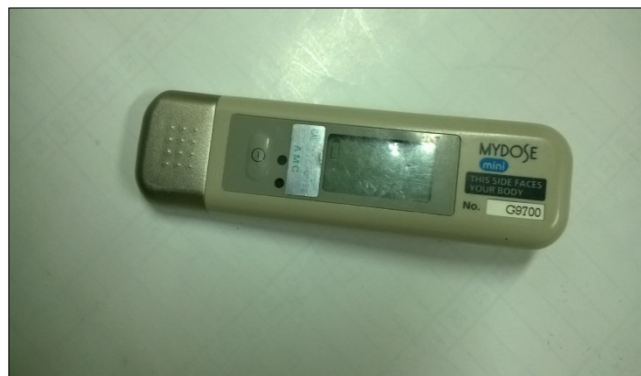
Figure 1. Showing dosimeter used to measure to absorbed dose of radiation.
