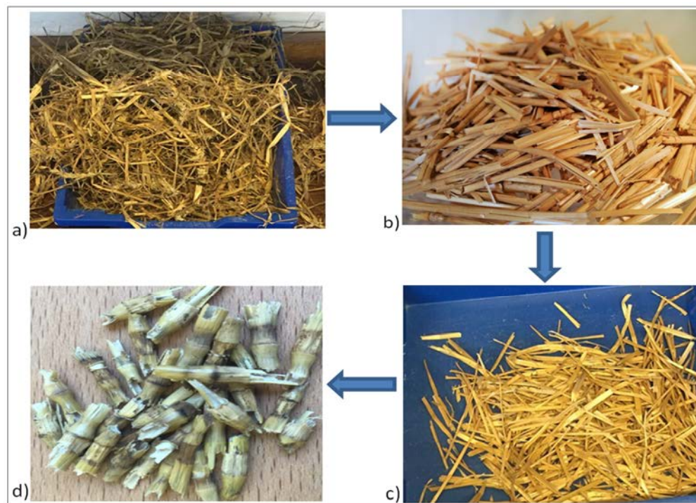
Figure 3. a) the separation of leave from stem of wheat straw, b) the straw stems cleaned, c) the internodes separated from the d) nodes.
