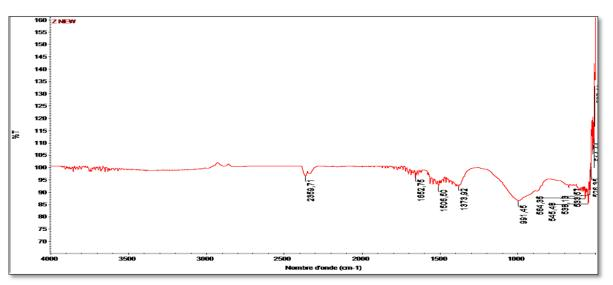
Figure 5. FTIR spectrum of Zn nanoparticles synthesized by *Portulaca oleracea L* leaves aqueous extract.
