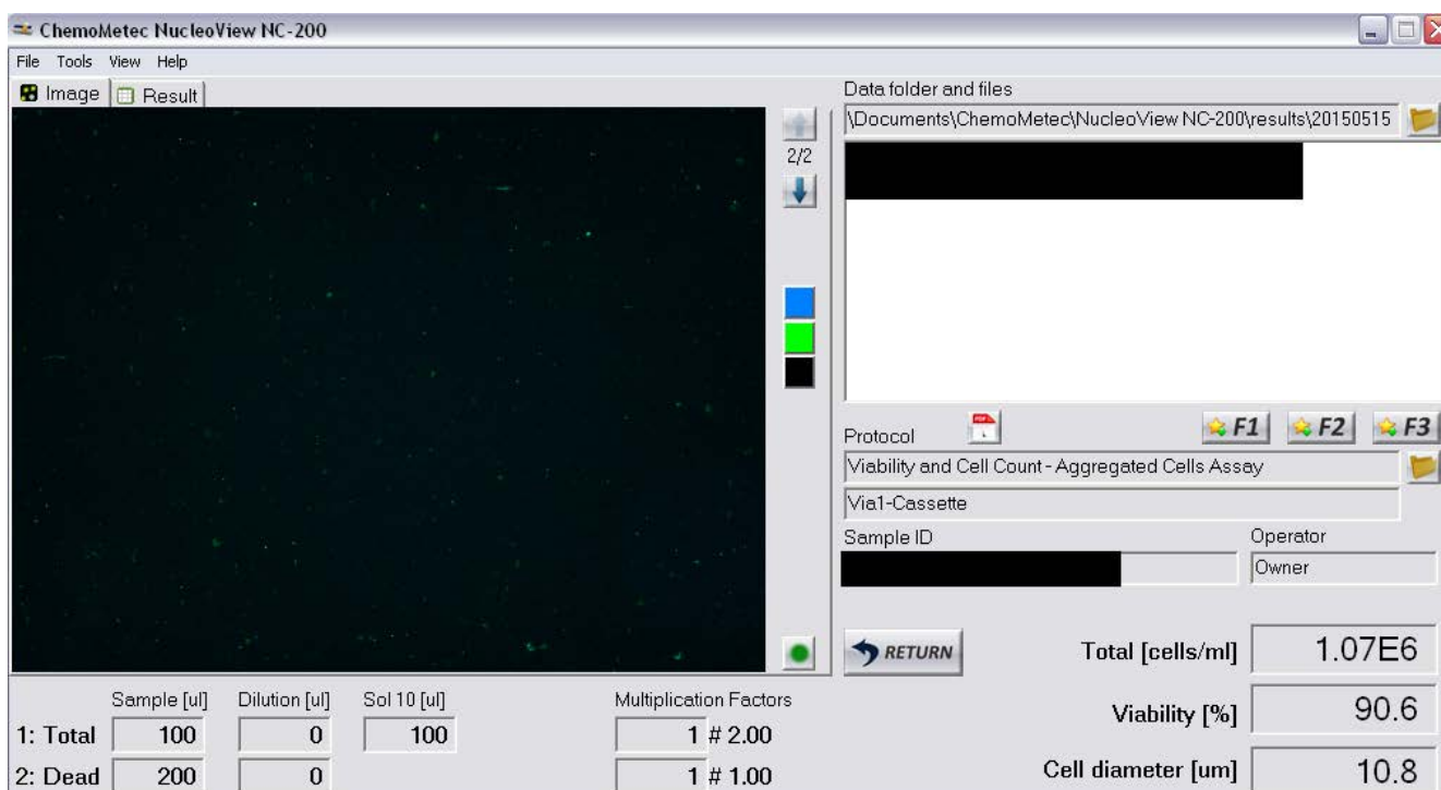
Figure 3. A representative readout from the Chemometec Nucleocounter NC-200. The sample tested was a 10% dilution of the final SVF output. The final volume of SVF was 12 mL total. 400 mL of lipoaspirate was processed. The total nucleated cell count for the whole SVF sample was 128.4 million nucleated cells. 321,000 nucleated cells were isolated per mL of washed lipoaspirate processed with 90.6% viability.
