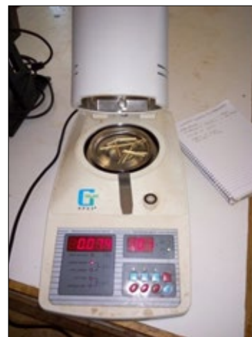
Figure 2. Infrared Moisture Genis Photometer (direct moisture tester).
