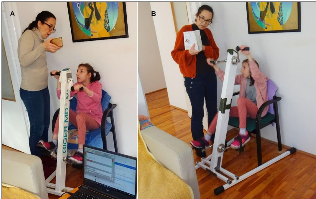
Figure 110. Layout of coordination dynamics measurements. The mother had to read aloud from a book (B) or show a video film on the smart phone while Anna was turning (A). Anna turns on a special CDT device type 1 (A) and type 2A (prototype) (B).
